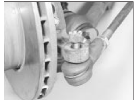
13.3 Track rod end balljoint nut unscrewed
