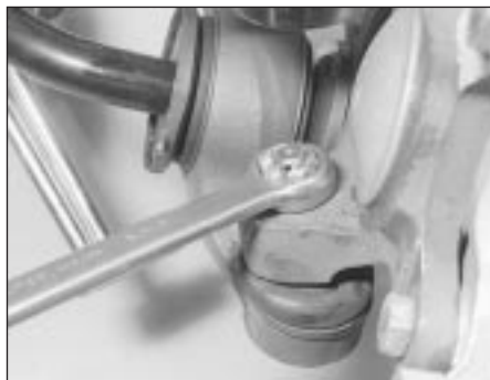
16.4 Slackening the front suspension lower arm balljoint nut
