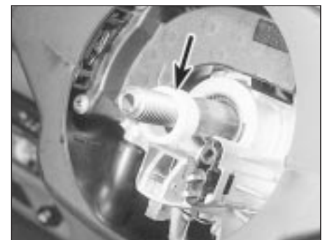
5.6 Spacer ring (arrowed) fits below steering wheel
