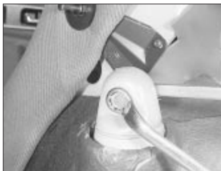
31.4 Undoing a rear shock absorber top mounting
