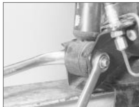
31.5 Undoing a rear shock absorber lower mounting
