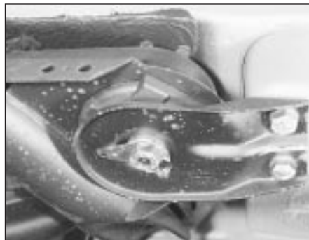
23.10a One of the rear suspension guide plates
