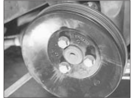
11.10 Unbolt the power steering pump pulley . . .
