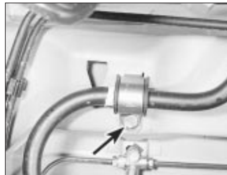
30.3 A rear anti-roll bar bracket - bolt arrowed
